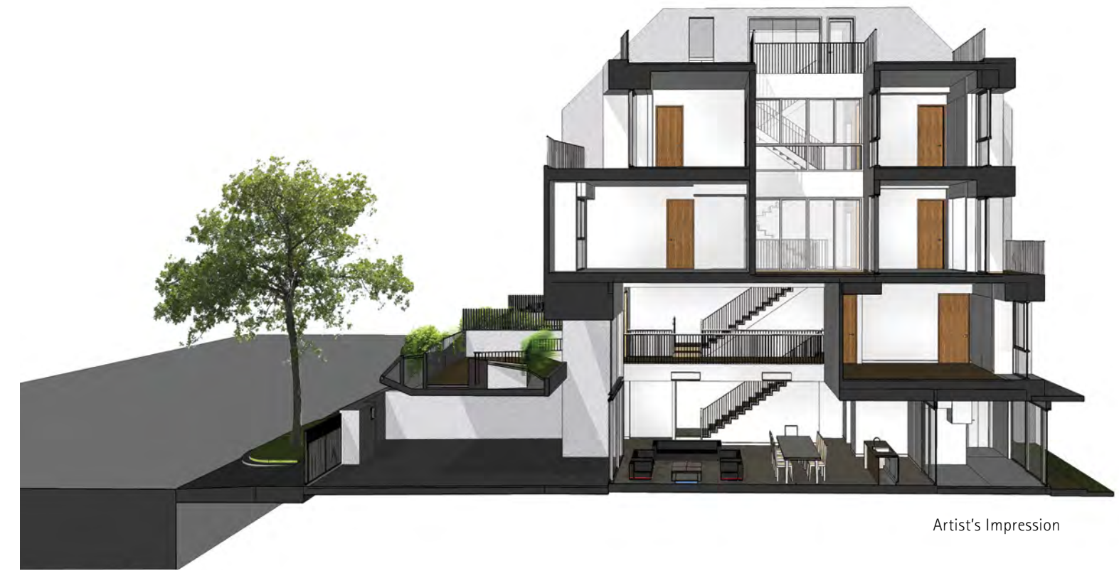
A cross-section of the interior and exterior layout of a typical Terrace House
